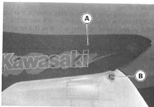
B. Seat Mounting Bolt
