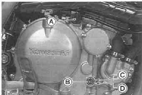
A. Oil Filler Cap C. Upper Level B. Oil Level Gauge D. Lower Level
